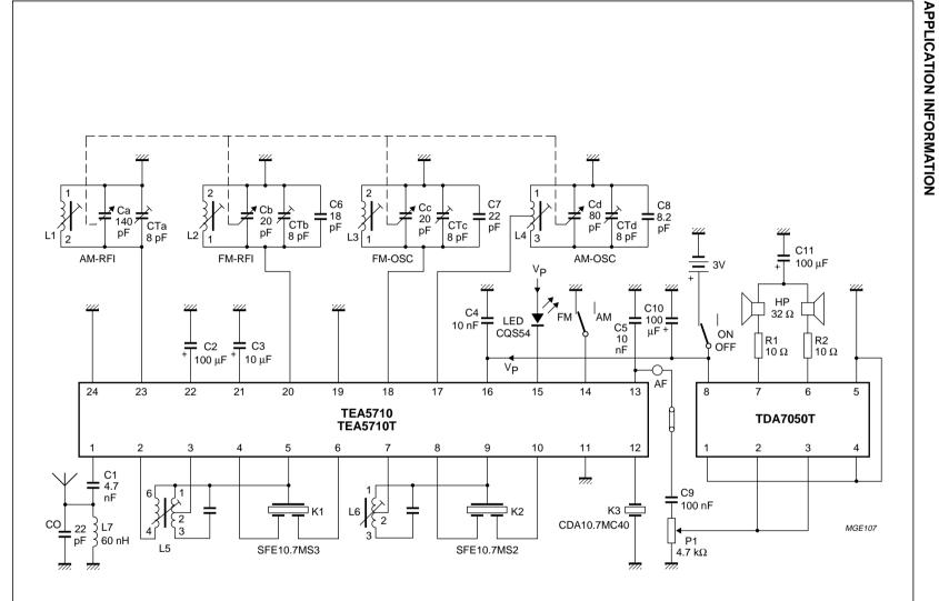
Fig.5 Application circuit of TEA5710 (AM: 522 to 1611 kHz, FM: 87.5 to 108 MHz) with stereo headphone amplifier TDA7050T.
