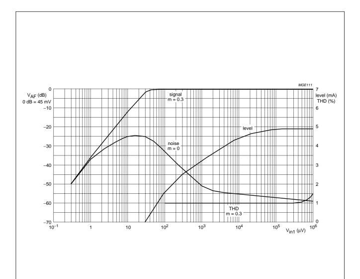
Fig.8 Typical AM audio output voltage ( $V_{AF}$ ; signal at m = 0.3), noise, THD (at m = 0.3) and indicator current (level) as a function of RF input voltage ( $V_{in1}$ ; f = 1 kHz). Measured in test circuit of Fig.4 with  $V_P$  = 3.0 V.
