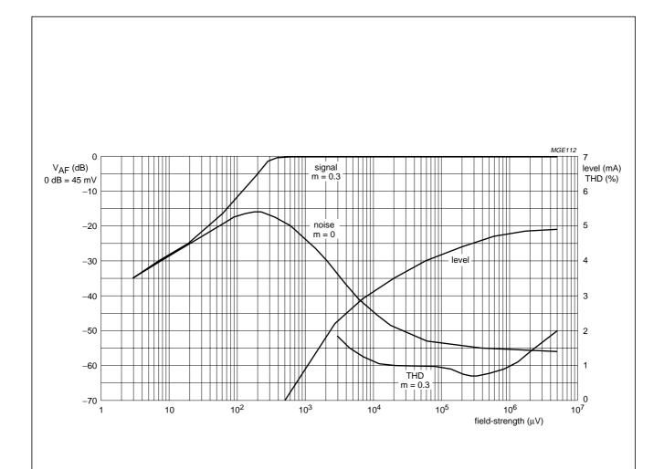
Fig.9 Typical AM audio output voltage ( $V_{AF}$ ; signal at m = 0.3), noise, THD (at m = 0.3) and indicator current (level) as a function of field-strength (f = 1 kHz). Measured at 1 MHz in application circuit of Fig.5 with  $V_P = 3 \text{ V}$ .
