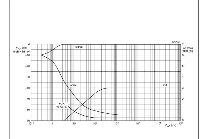
Fig.10 Typical FM audio output voltage ( $V_{AF}$ ; signal), noise, THD and indicator current (ind) as a function of RF input voltage ( $V_{in3}$ ;  $d_f = 22.5$  kHz). Measured in test circuit of Fig.4 at  $V_P = 3$  V.
